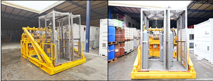
TWIN BASKET LAUNCH AND RECOVERY SYSTEM
