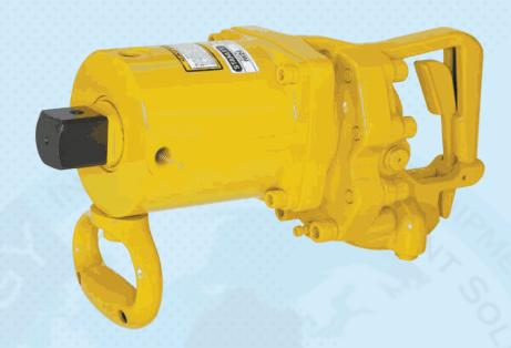
The Stanley **IW24** is an extreme heavy duty 1½" square drive impact wrench designed for the toughest underwater bolting applications. Powered by a Stanley integral Hyrevz motor, the **IW24** has a durable swing hammer impact mechanism with adjustable impact intensity from 800 to 3500 ft lbs (1088 to 4760 Nm) of torque.
